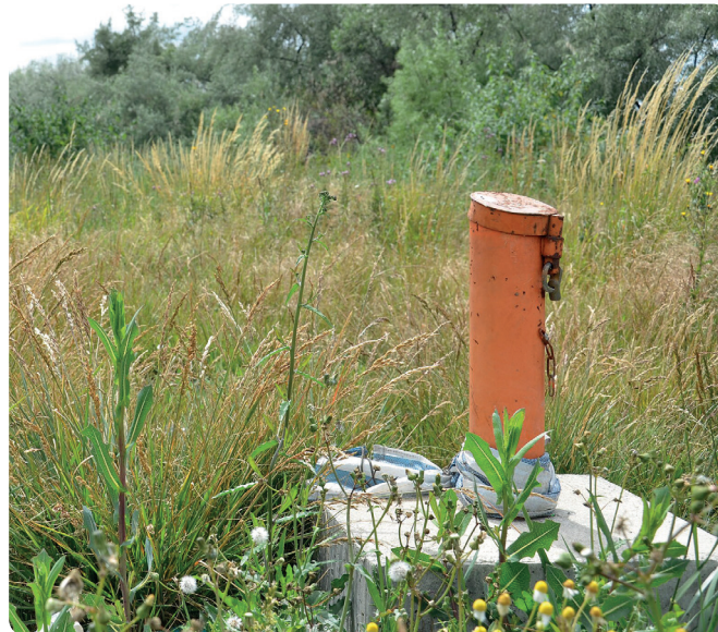
The flow and level of groundwater are monitored particularly through measurements provided by piezometers.
